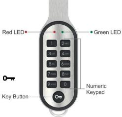
4. Insert the drive into a computer within 30 seconds of unlocking. It will now allow continuous use until it is locked once again. If the drive is not inserted in the allotted time, it will automatically lock and will have to be unlocked again in order to use.
